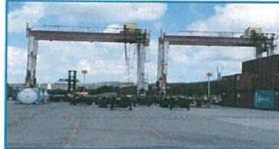
Rubber-Tired Gantry Cranes
