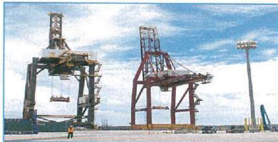
Gantry Cranes 2 and 3 have been decommissioned due to its deteriorating condition and have come to the end of their safe working lifespans.
