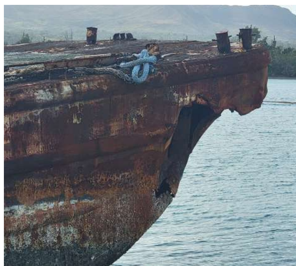
The YFN-816 barge located at F6 is seen in this recent photo with a significant hole. Contractors were able to refloat the barge to prepare for the removal next month.
